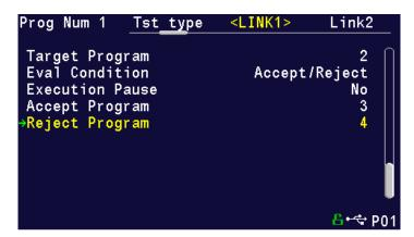
The second link required by the example above targets Program 3. If Part 3 is Reject, then Program 5 will run. If Program 3 is Accepted, the test sequence stops with a Program Accept light and a Program Accept.
