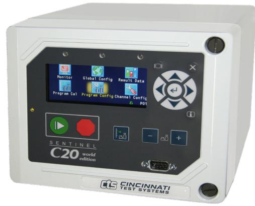
Sentinel C20 leak test instrument
