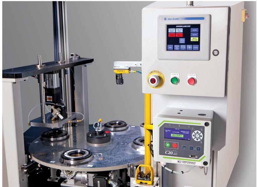
C20 integrated into an automated test cell
