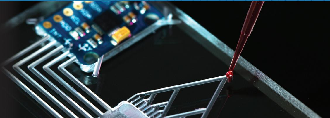
Microfluidic chips are used in a multitude of biological diagnostic applications, including analytical separation, detection, fluid control (sampling/mixing) and more. Once placed within durable analytical instrumentation, these devices typically have multiple unique micro pathways isolated from one another for liquid media passage, sampling and analysis.
