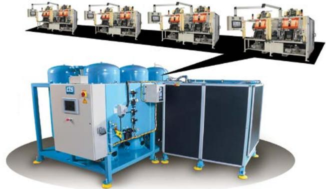
**CTS Helium Reclaim System recycling test helium from a line of Custom Hard Vacuum Helium Test Machines**
