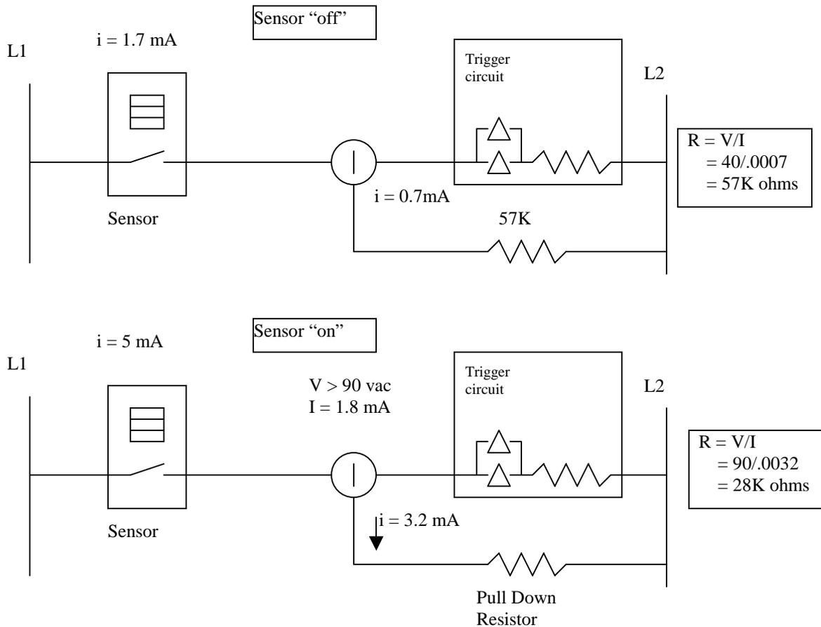
Note that this particular sensor has a “minimum load current” requirement, so we are obligated to use as 28K or smaller resistor. To be safe, we would choose a 20K resistor, which would have to dissipate  $(120)^2/20,000 = 0.72$  Watts. A 1 Watt resistor will get very hot dissipating this much heat. You need to plan accordingly.
