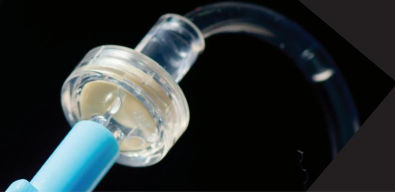
Check or one-way valves allow liquid flow in one direction and resist reflux, or back-flow, in the opposite direction based upon the presence of an internal elastomeric “duckbill” valve or an elastomeric disc. This elastomeric valve is often housed in an injection-molded polymer/plastic body which is either ultrasonically welded or adhesively bonded.
