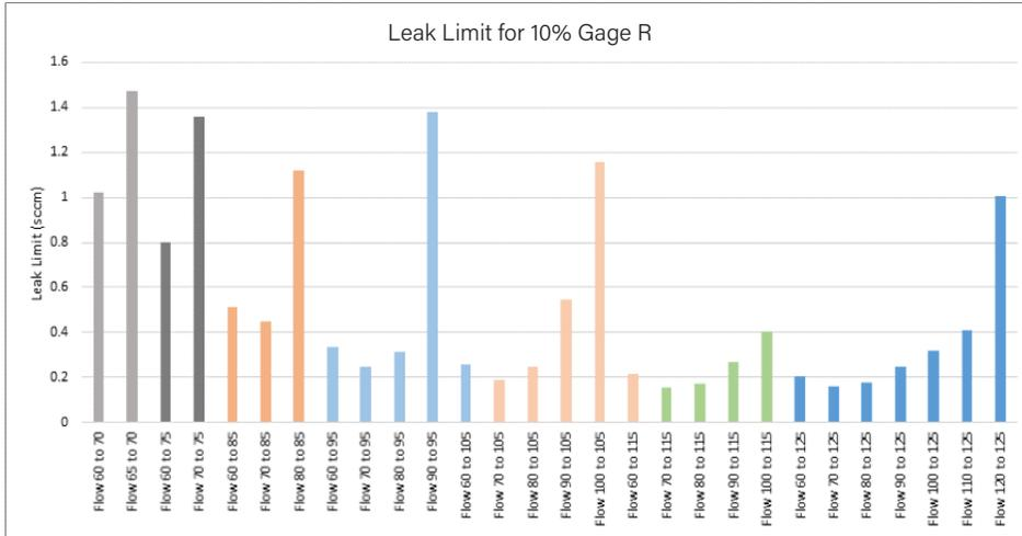
This graph, produced using Sciometric's QualityWorX data analysis tools, shows a comparison of leak rate vs. gage R with gage R constant at 10%. This data enabled the manufacturer to clearly see the impact of shortening cycle time and how it would affect the leak rate and the gage R.
