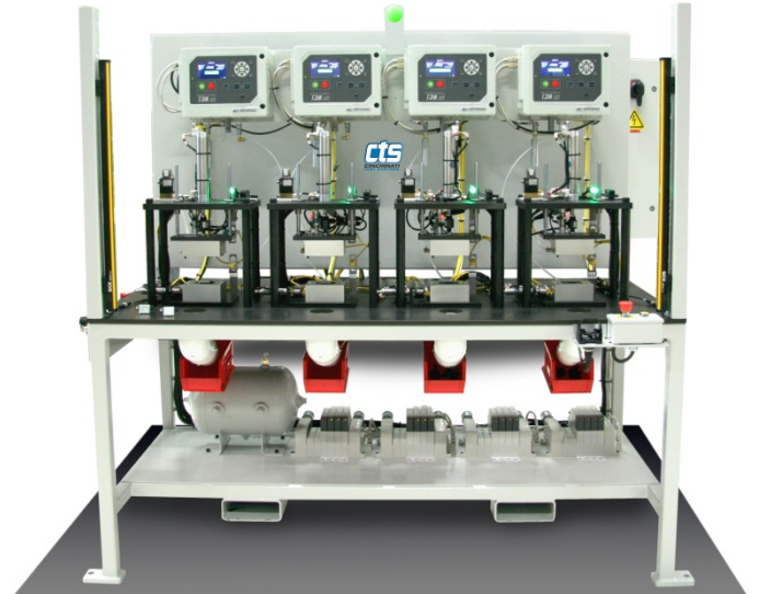
Four Station Test System designed to individually test sealed electronic sensors
